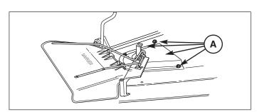
Figure 2. Install Discharge Baffle A. Cover and Bolts
